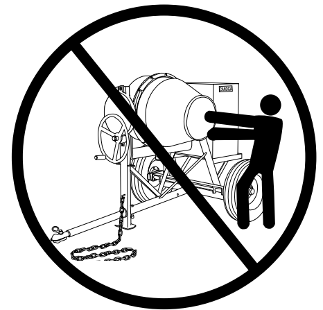
Fig 14. Filling Mixing Drum
